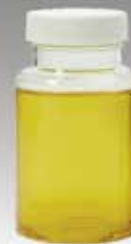
Yellow is positive for total coliforms.
