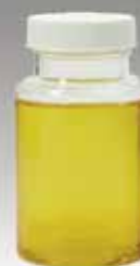
Yellow is negative for total coliforms and E. coli .
