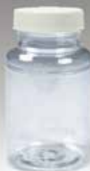
Clear is negative for total coliforms and E. coli .
